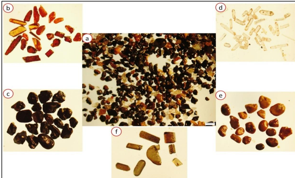
Fig. 11. Stereo microscopic image showing: a – heavy mineral fraction content, b – rutile, c – ilmenite, d – zircon, e – leucoxene, f – green silicates
