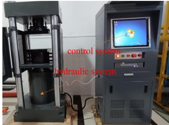
Fig. 3. Microcomputer-controlled servo hydraulic pressure testing machine
