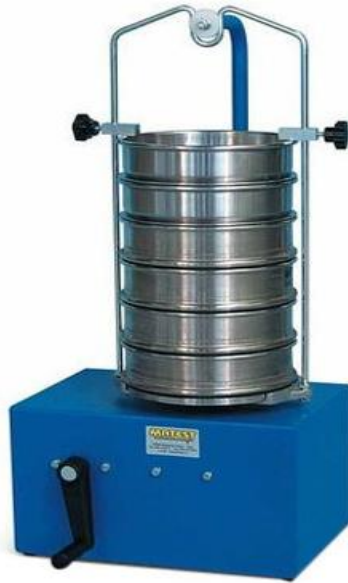
Fig. 11. Sieve Shaker set up for the present investigation
