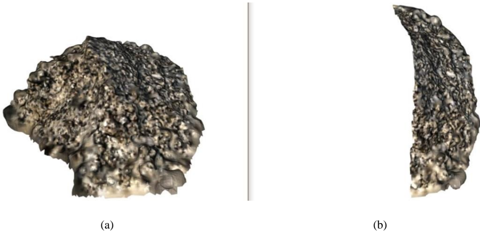
Fig. 22. 3D reconstructed model of overburden heap: (a) final mesh surface of the 3D reconstructed model, and (b) a cross-sectional view of the 3D reconstructed model showing the 2D profile
